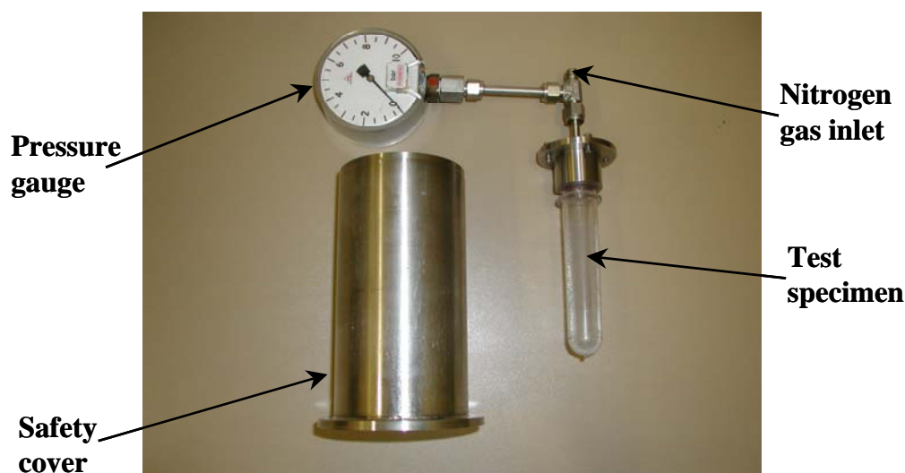
Figure 1 Chemical probe instrumentation designed for use with bottle preforms.
